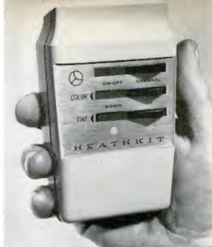
WIRELESS REMOTE CONTROL turns set on and off, changes channels and adjusts volume and color—all from across room without your leaving your chair
